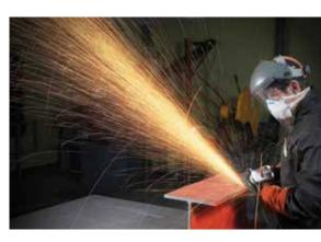
VATOR features an extra strong disc base/backing for more powerful and aggressive grinding action. It also features a patented UHR multi-layer manufacturing technology to prevent edge flakiness-keeping the wheel edge symmetrically round for more safety and longer life. For additional information visit Walter Surface Technologies at www.walter.com.
